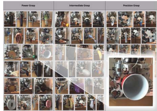
Fig. 15: Performance Test from the FFP Index. 62 out of 63 successfully performed prehensile grasping tasks
