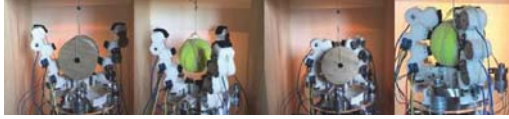
Fig. 12: Test setup for testing the payload for the cylindrical and spherical power grasps
