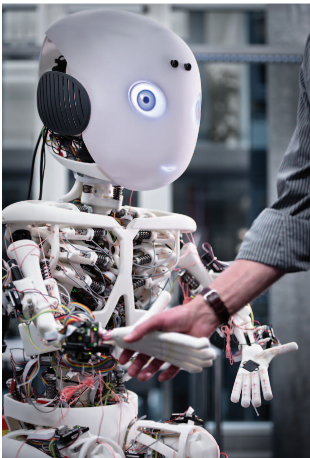
Figure 7. Roboy, a human-like, musculoskeletal robot with 28 degrees of freedom and 48 motors, to be controlled by brain-inspired systems. (Photograph courtesy of Adrian Baer.)
